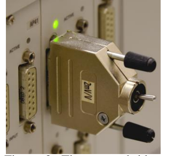
Figure 3: Three-state bridge as a voltage ratio transfer standard.
