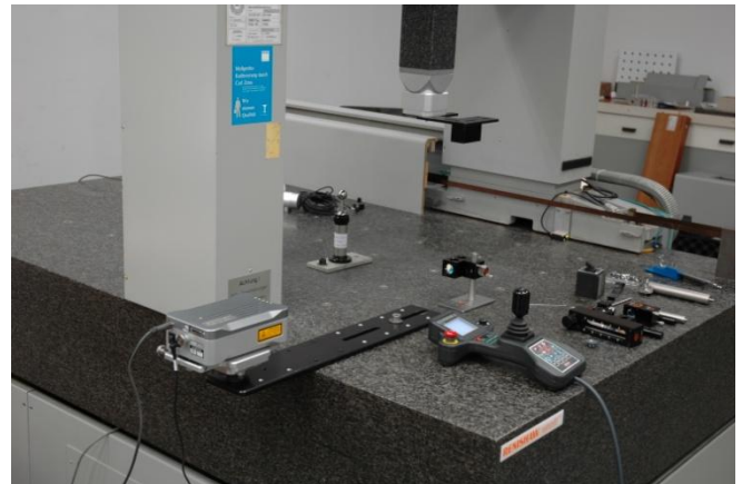
Fig. 2: Measurement of rotation errors using laser interferometer
